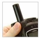
**5.** Press down on the protective cover to expose the handset's contacts.
