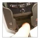
**6.** Slide the mating connector through the guide slot and 'click lock' with the handset.
