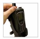
**4.** Rotate the handset lock to secure the handset.
