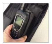
The dock is easily installed into the bag via a 'hook and loop' attachment. Ensure that the antenna attachments are secure. Antenna cables route through the bag internally to storage in the bottom of the bag.
