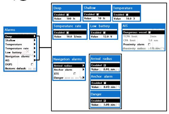
A warning message with beep sound is displayed when an alarm condition is met by user setting. Press to clear the alarm. However, the alarm will be displayed again when the alarm condition occurs again. The unit provides alarms for various functions.
