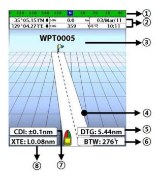
The **Highway** window shows a 3D view of the vessel traveling through the water when navigating to a destination point.
