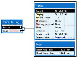
The unit has the capability to store 10 individual tracks and record up to 15,000 track points. Before using the track function you will need to setup the track function that suits your boat.
