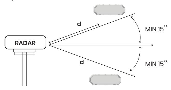
d = 2 meters for S-Band up to 50kW d = 4 meters for X & C-Bands up to 50kW
