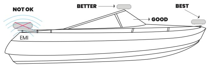
EMI (Electromagnetic Interference) from engine components
