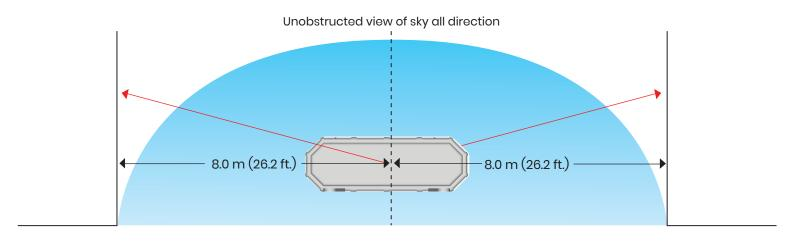
Keep the safe distance of Barracuda ADU from RADAR radiation
